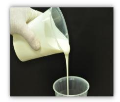
Polymer Polyol – One of the most important components used for some heavy duty applications such as low density moulded automotive seating, high resilience foams, hot or cold mold foams, RIM and integral skin.
